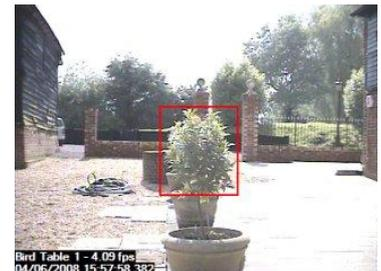
iCatcher has an intelligent masking ability that works much better than the simple masking employed by other systems. The ICE intelligent mask allows you to still ignore the areas you want to mask from false alarms but it will still **track moving objects** through the masked areas.
