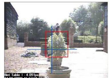
The image on the right shows on object that originated from outside the mask is still being tracked and recorded as it passes through the masked off area.
